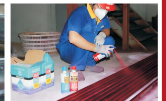
无损探伤Liquid penetrate Test
